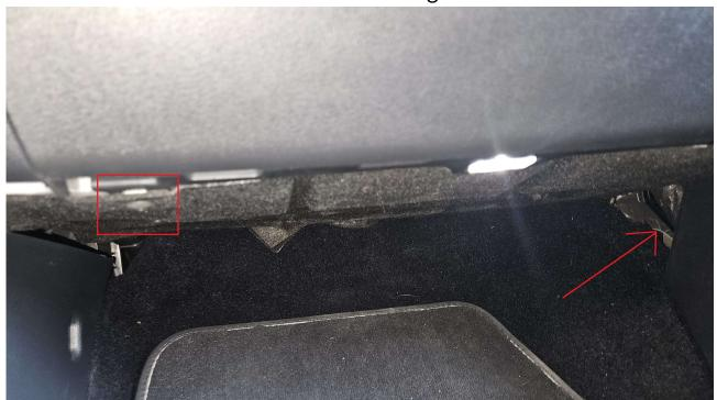
3. The control unit is located at the bottom of the passenger side A pillar:
